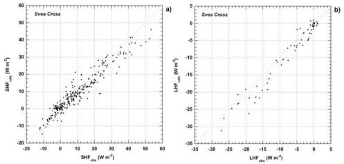
Figure 1: Comparison of calculated and measured SHF (a) and LHF (b) at AWS 6 (situated at 'Svea Cross') for a summer period in January 1998.
