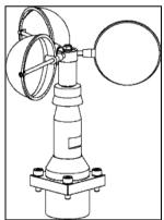
Figure 5: A custom anemometer design uses bearings that remain operational to -60 °C.
