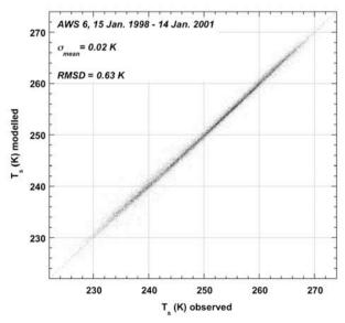
**Figure 2:** Scatterplot of 'measured' (derived from LW $\uparrow$ ) and modelled surface temperature T<sub>s</sub>, based on two-hourly averages for a four-year period.
