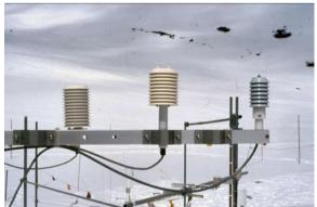
Figure 1: Radiation shields used in the experiment: Young (left), Mierij (middle), Aanderaa (right).
