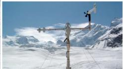
**Photo:** The IMAU AWS on the Morteratsch glacier. (Photo: Dieter Scherer)
