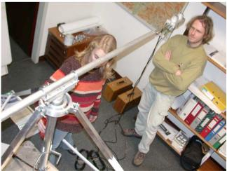
Figure 2: The cardan-like joint is the core of the self-adjusting mounting device (Foto: G. Kaser).
