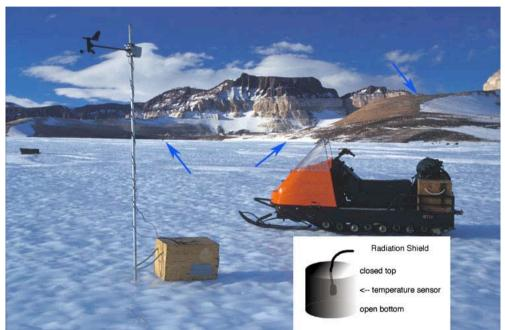
**Figure 2:** This picture shows one of the Davis weather stations in January 2003. The locations of three other stations are indicated by the arrows. The inset shows the design of the radiation shield used for the Davis temperature sensors.
