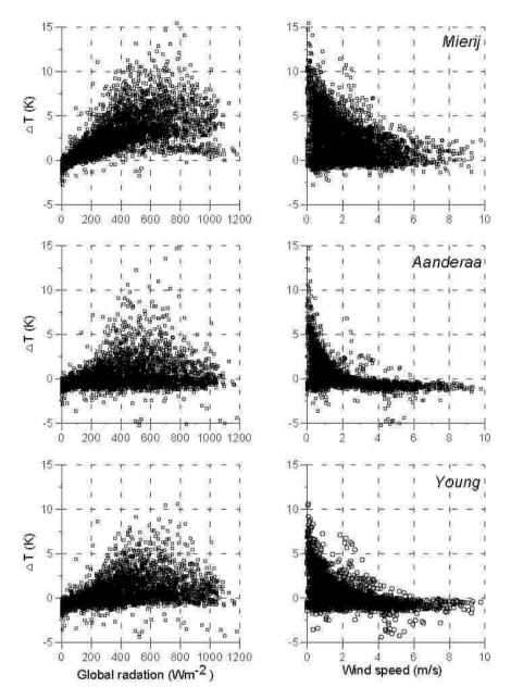
Figure 3: Differences between unventilated and ventilated air temperatures (10-minute averages) versus global radiation and wind speed.
