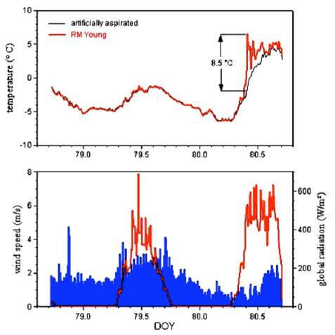
**Figure 1:** Measurements of temperature in an artificially aspirated (Kroneis 430M) and in a plate shielded (R.M. Young) device. The lower panel indicates wind speed and global radiation as measured at the site (Obernberg, 1999).
