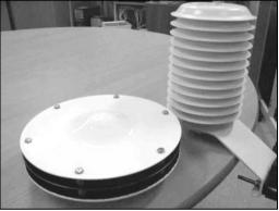
**Figure 4:** A Climetrics' screen beside a Young highlights the move away from an approximation to a Stephenson screen made by the three-plate design. The blackened internal plate surfaces reduce internal reflections whilst the metal plates provide improved thermal coupling.
