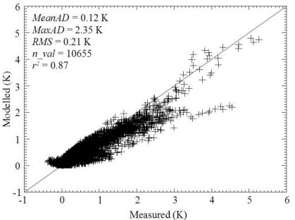
Figure 4: Comparison of modelled and measured temperature differences for the whole measurement period.
