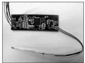
**Figure 2:** Precision temperature sensor interface and NTC thermistor. The intelligent sensor interface is used, with some transducer interface modifications, on all Climetrics' sensors.
