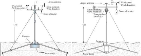
Figure 1: Schematic figures of the first 2 types of weather stations deployed by the IMAU.
