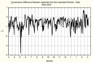
Figure 4: Mean daily temperature difference, ventilated vs. non-ventilated.
