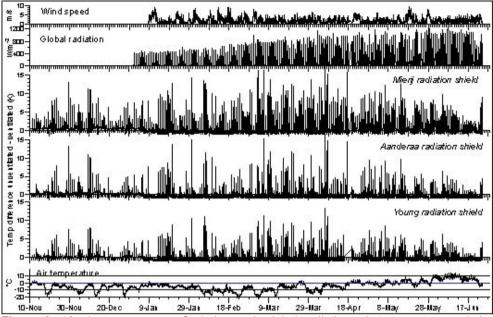
**Figure 2:** 10-minute averages of wind speed, global radiation, air temperature and the difference between unventilated and ventilated air temperature using three different types of radiation shields at Weissfluhjoch, Davos, from 10 Nov 1995 – 18 June, 1996.
