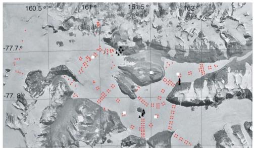
**Figure 1:** Location map of stations on the Taylor Glacier, Antarctica. Red circles are movement and ablation survey poles. Black triangles show the location of temporary weather stations we set up in the austral summer 2002-3. White squares show the location of permanent weather stations we set up in the austral summer of 2003-4.
