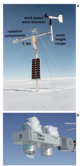
**Figure 2:** a) picture of AWS 9. The data logger and pressure sensor are buried in the snow; b) enlarged image of K&Z CNR1 radiation sensor.
