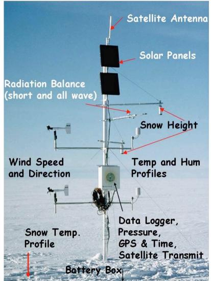
Figure 1: GC-Net automatic weather station instruments.
