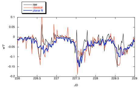
**Figure 2:** Sensible heat flux as measured by the sonic anemometer (raw) (ms-1K), and after tilt correction using the classical and the planar fit method. The data are for three summer days in 2002.
