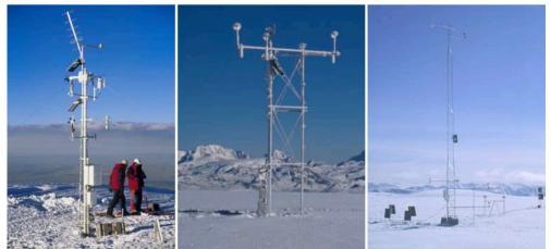
Figure 1: AWS on Sajama (left), Quelccaya Ice Cap (center), and Murray Ice Cap (right).
