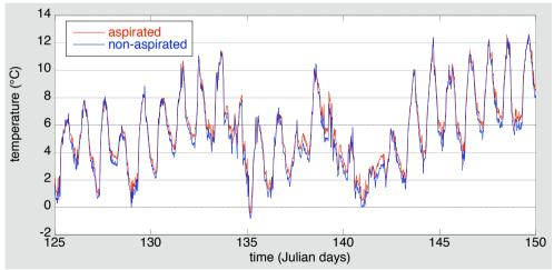
**Figure 4:** A comparison of temperature measurements (30-min values) with an aspirated and a non-aspirated instrument. The sensors were placed on different masts a few m apart. Height of the instruments: about 3.5 m.
