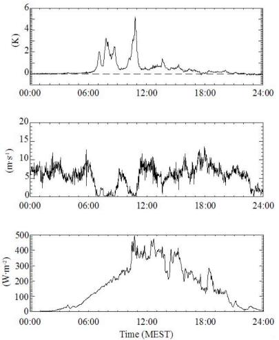
**Figure 2:** Differences between minute values of Vaisala HMP 35A and psychrometer air temperatures (upper graph), and their dependencies on wind speed (middle graph) and upwelling short-wave radiation (lower graph), measured on May 30, 1998.
