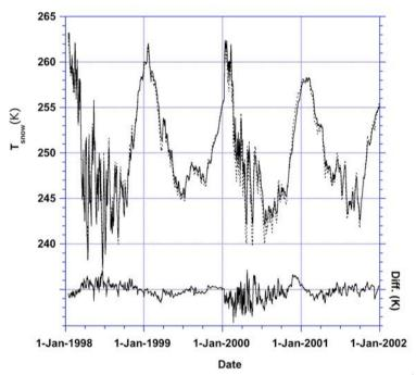
**Figure 4:** Measured and modelled snow temperature (upper lines) and the difference (lower line). Depths of snow temperature sensors ranges from 0.2 to 2 m.
