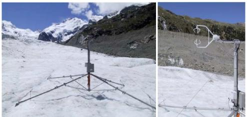
Figure 1: Sonic anemometer on the tongue of Morteratschgletscher.
