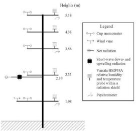
**Figure 1:** Instrumentation used during the field campaign in the Kärkevagge, Swedish Lapland, during the snowmelt season in 1998.
