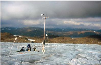
**Figure 2:** The IMAU-AWS on Hardangerjökulen, Norway, in September 2000 (photo by Wim Boot). The mast has four legs and stands freely on the ice. The mast is about 6 m high. Two sonic rangers are used: one on a tripod drilled in the ice (8 m stakes), and one in the mast (below the Young anemometer).
