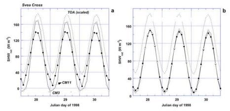
**Figure 3:** a) SHWnet for three days of fair weather at Svea Cross, as measured with the Kipp and Zonen (K&Z) CM3 and K&Z CM11. SHW↓ at top-of-atmosphere (TOA) is also shown, scaled and offset for comparison; b) same as above, but after correction using the method of 'accumulated albedo'.
