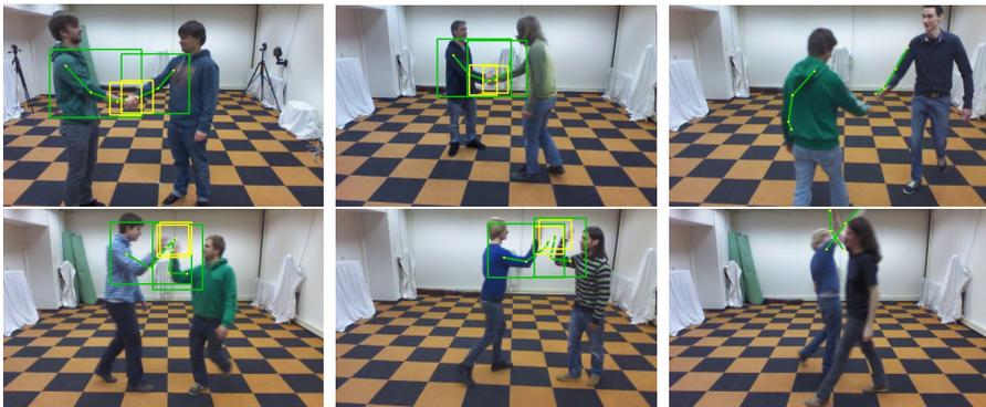
Fig. 2: Processed frames with respect to a seed frame (left): one with low (middle, both  $RE = 0.15$ ) and one with high (right,  $RE = 0.81$  and  $RE = 0.52$ ) residual error. The bounding boxes are omitted in the rightmost images because they are not used for poselet creation, as the residual error exceeds the threshold.
