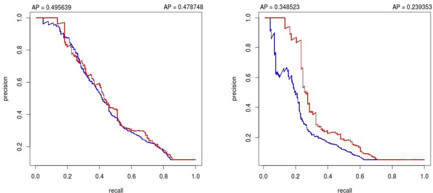
Fig. 8: The precision-recall diagrams for hand shake (left; red line, 0.75/0.25:  $AP = 0.50$ ; blue line, 0.25/0.75:  $AP = 0.48$ ) and high five (right; red line, 0.75/0.25:  $AP = 0.35$ ; blue line, 0.25/0.75:  $AP = 0.24$ ).
