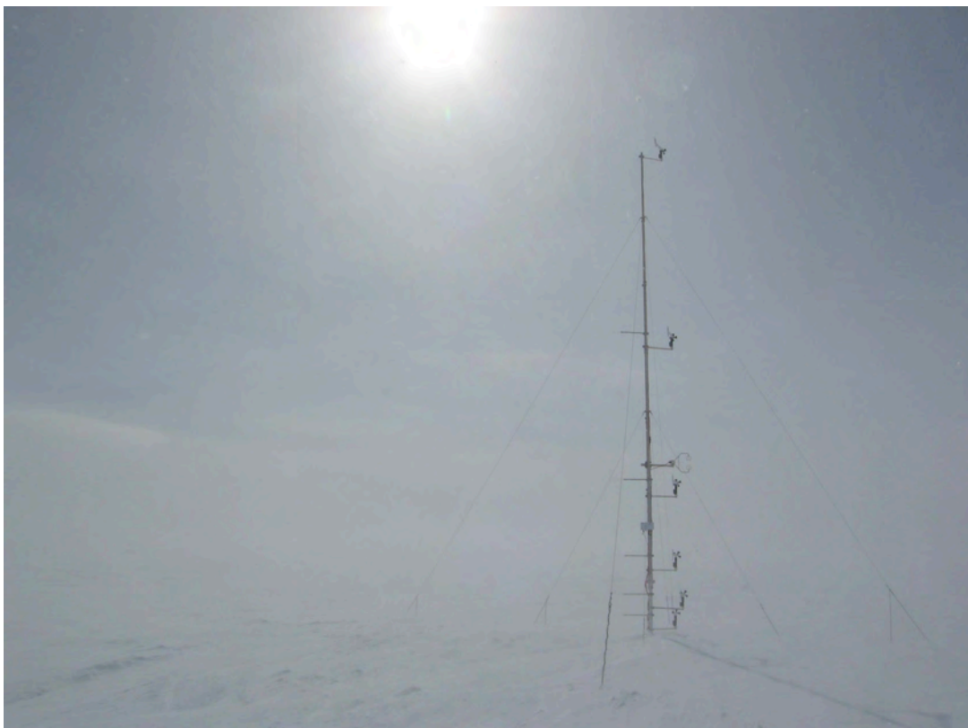
Figure 8. The profile mast and sonic anemometer at the location of AWS 5 during blowing snow conditions. Photo by Paul Smeets.
