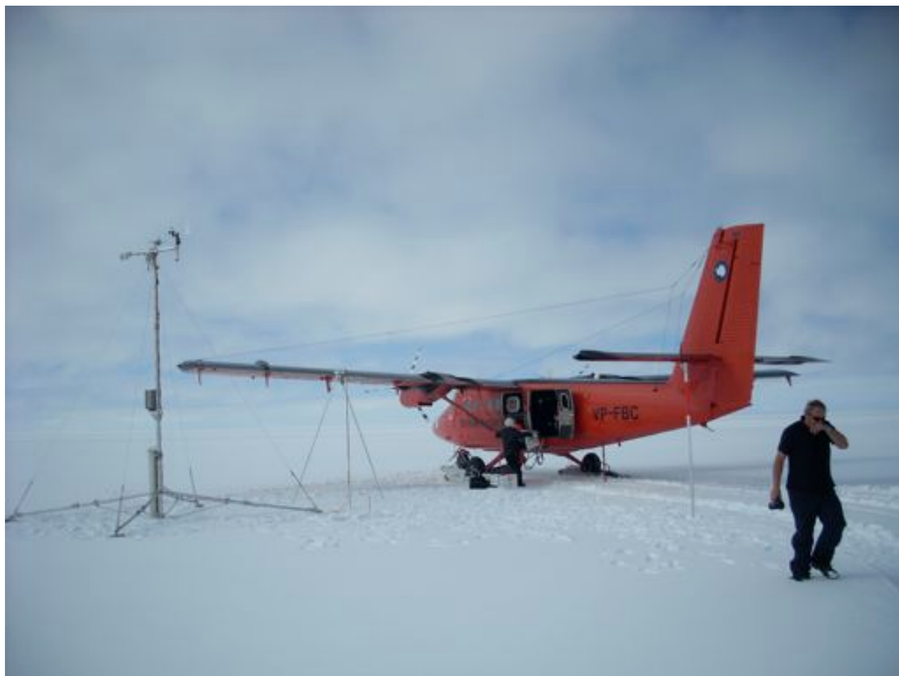
Figure 9. The completed AWS15 on Larsen C ice shelf, next to the BAS Twin Otter. Right of the AWS a stand-alone height sensor is installed as well as a stand-alone GPS receiver (with red tape for enhanced visibility), with ARGOS antenna.
