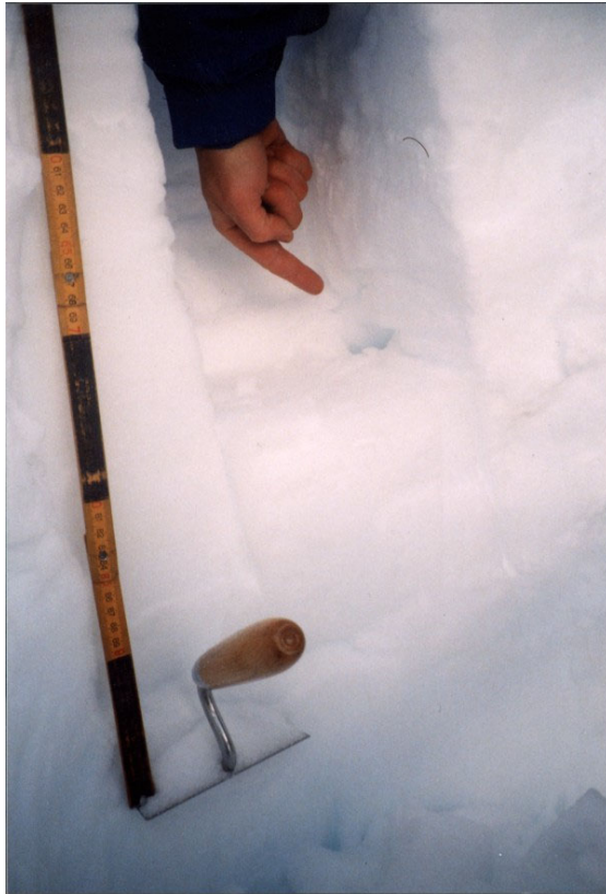
Figure 7: Snow pit at AWS 6, finger pointing at a hollow space in the snow pack (photo: Dan Zwartz).
