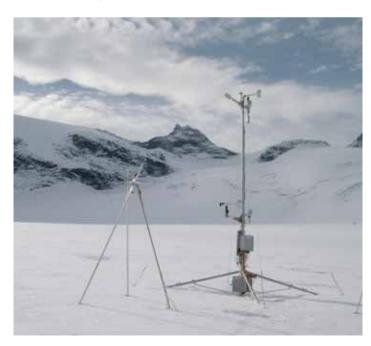
Figure 1. The automatic weather station Storbreen. Norway. Measurements humidity. temperature and wind are done at two levels.about 2 m and 6 m above the ice surface.The free standing sonic ranger (to the left) measures ice melt and snow accumulation. Photo: Liss M. Andreassen.
