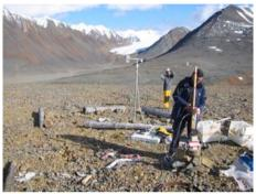
**Figure 3.** Meteorological station at No.31 Glacier. Thermometer, anemometer, solar radiation meter and snow-depth camera were installed.
