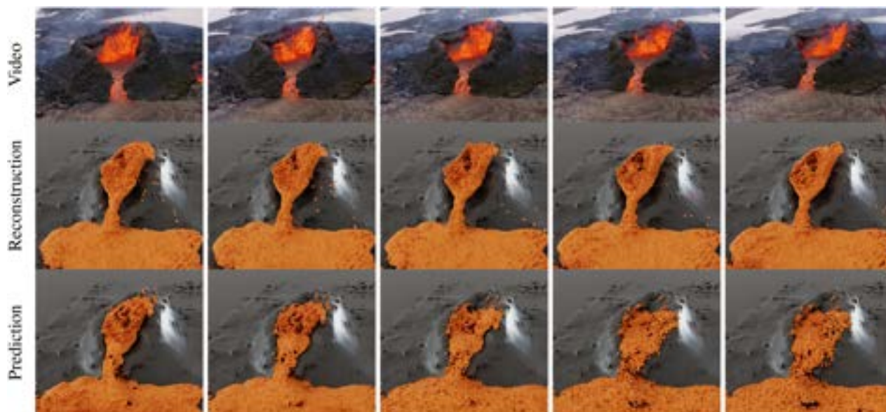
FIGURE 10 | Particle reconstruction and fluid prediction on the real-world Lava test set. The first row shows the original video, the second row shows corresponding fluid particles reconstructed from the video, and the third row shows fluid predictions after the video.
