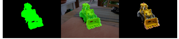
Figure 8: Projected mask on the input viewpoint to create a segmentation mask of the OOI.
